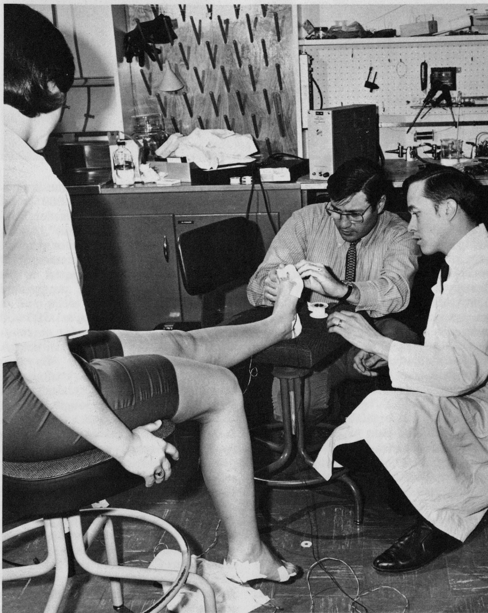
Dr. Morris Milner (left) and Arthur Quanbury attach footswitch electrodes to the foot of a subject at the start of a gait characteristics study.
